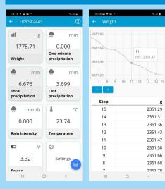
Scan for nearby compatible sensors. Display current measurements. Display short-term measurement history in grafical and tabular form. Change sensor setttings. Upload firmware.
