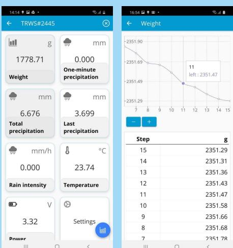
Scan for nearby compatible sensors. Display current measurements. Display short-term measurement history in grafical and tabular form. Change sensor setttings. Upload firmware.
