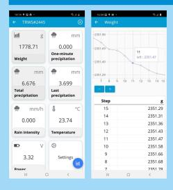
Scan for nearby compatible sensors. Display current measurements. Display short-term measurement history in grafical and tabular form. Change sensor setttings. Upload firmware.
