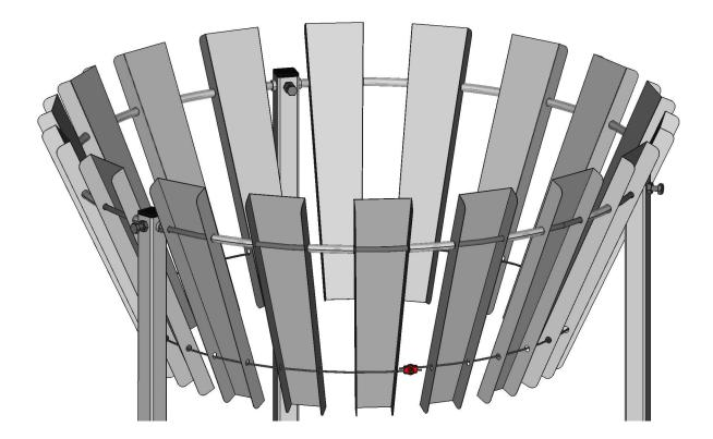
• Connect both ends of the cable using the provided clamp. Tighten with a 7 mm socket wrench.
